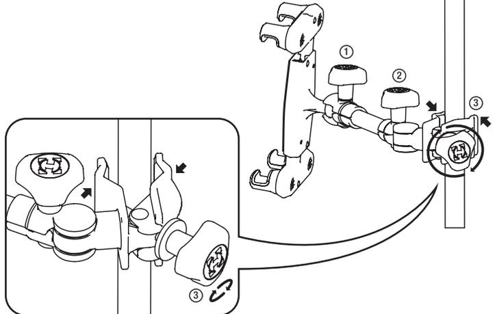
Loosen/ tighten the knob (3) to mount to the pole.
