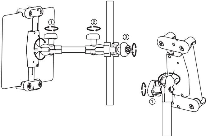
360° balljoint adjusts your device to desired positions by loosening the knob (1&2).
