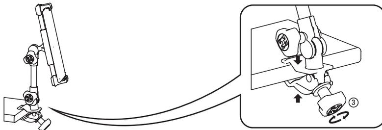
Loosen/tighten the knob (3) to attach onto the desk (less than 3 cm/1.18" thickness).
