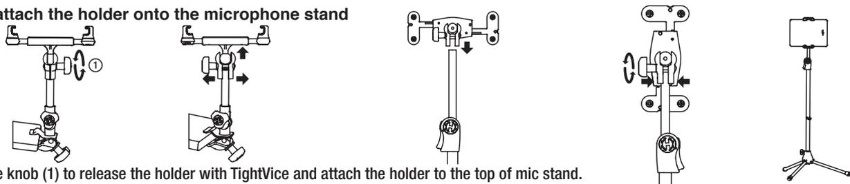
Loosen the knob (1) to release the holder with TightVice and attach the holder to the top of mic stand.
