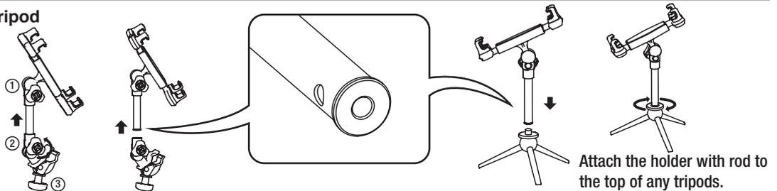
Loosen the knob (2) to release the holder with rod and find the 1/4"-20 threaded hole on the rod's bottom.
